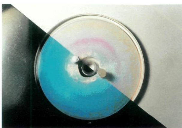
Figure 2. (a, top) Photograph showing a rotating observation cell. D1B72 suspension 5 days after the sample was set. [D1B72]_0 = 0.0820 ; Close-up picture was taken with an acute angle illumination. (b, bottom) Photograph showing the observation cell on black and white color papers. After the reflection spectra were taken at the centrifugal equilibrium, the cell was detached from the driving motor and the close-up picture was taken with zero angle illumination.
