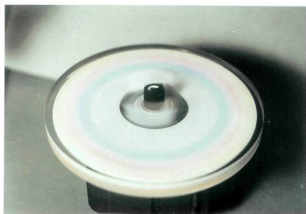
Figure 1. Photographs showing the rotating observation cell. D1K88 suspension 5 days after the sample was set. [D1K88]_0 = 0.0617 in volume fraction. (a, top) Close-up picture was taken with an obtuse angle illumination, (b, bottom) Close-up picture was taken with an acute angle illumination.
